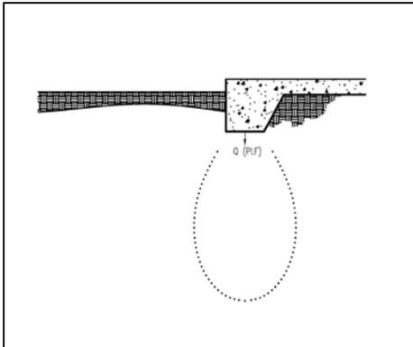
Determining a reasonable depth for the zone of influence is required during the design phase of construction projects to estimate the amount of settlement a structure may undergo due to the proposed change in loading to the subgrade. This method commonly known as the Boussinesq ['bü·si'nesk] method is widely used throughout the geotechnical industry. In addition to estimating the settlement of structures supported on shallow foundations
